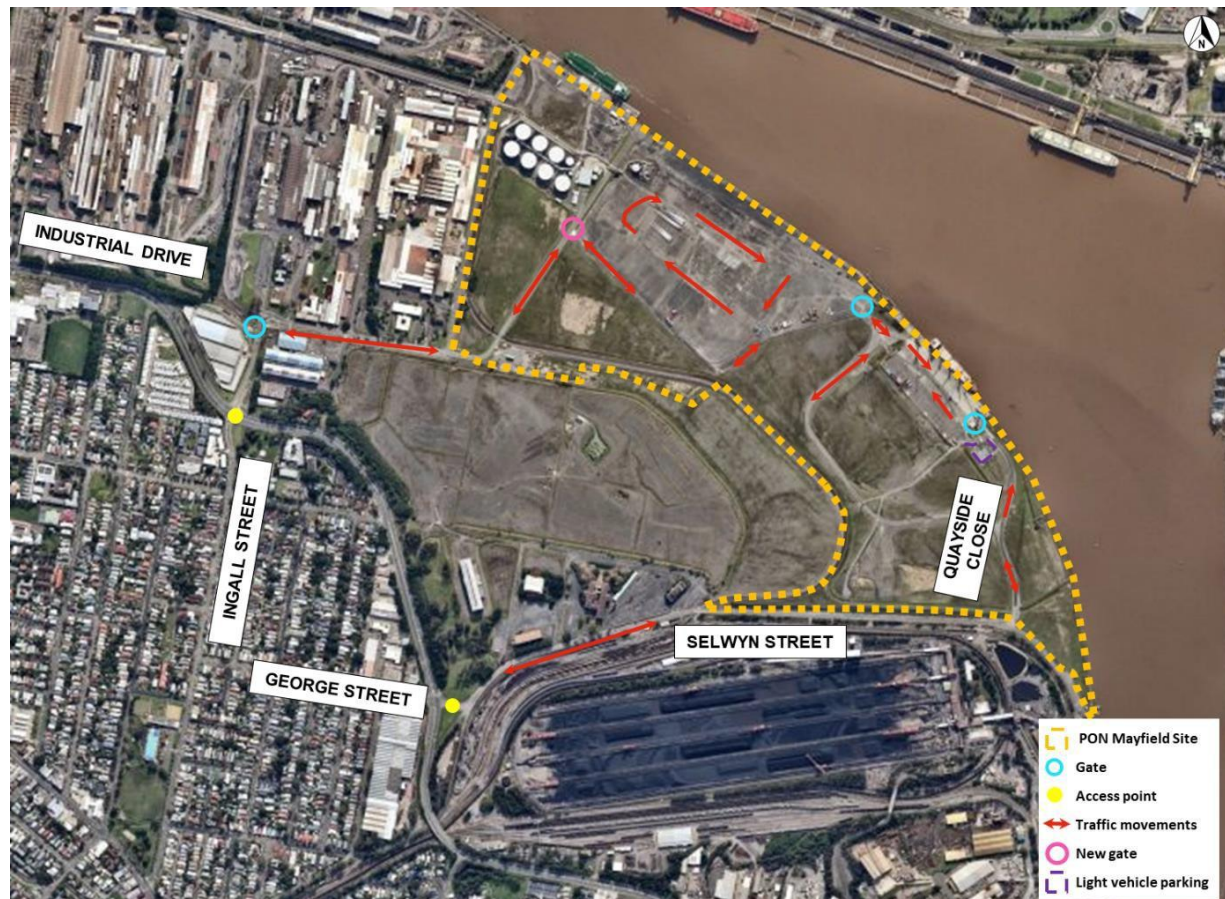
Figure 2-2 PON access and traffic movement network
